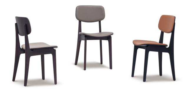
LEAF / FRAME & SEAT: Seat and Backrest are constructed with curved plywood and covered with integrally-molded polyurethane foam. Frame is comprised of solid ash wood, available in Black Walnut or Brown Walnut finishes. LEGS: Capped with Teflon glides. UPHOLSTERY: Available in Leather only. Covers not removable.
